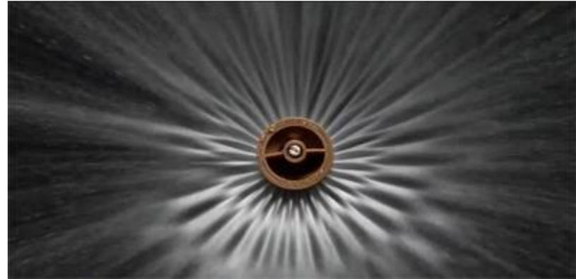
Rainbird HE-Van nozzles – matched precipitation any arc, any radius 1.5-1.7"/hr @ 30 psi
