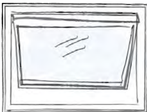
Awning window A window that is hinged at the top and swings outward.
