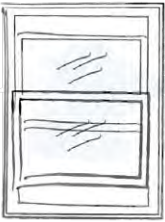
Double-hung window A window with upper and lower sashes that operate independently.
