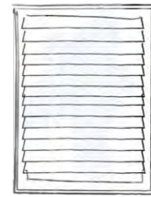
Jalousie window A window composed of angled, overlapping slats of glass, arranged horizontally like a shutter to tilt open.
