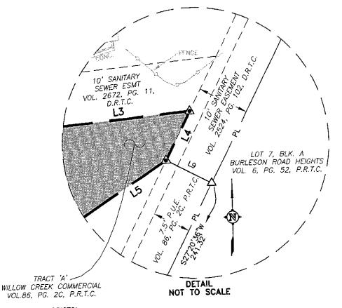
**LEGEND** 1/2" IRON ROD FOUND (UNLESS OTHERWISE NOTED) ◬ 60D NAIL SET CALCULATED POINT Δ 60D NAIL FOUND P.O.B. POINT OF BEGINNING RIGHT-OF-WAY R.O.W. PROPERTY LINE — PL — PUBLIC UTILITY EASEMENT P.U.E. TRAVIS COUNTY APPRAISAL DISTRICT T.C.A.D. VOL., PG. VOLUME, PAGE DEED RECORDS OF D.R.T.C. TRAVIS COUNTY
