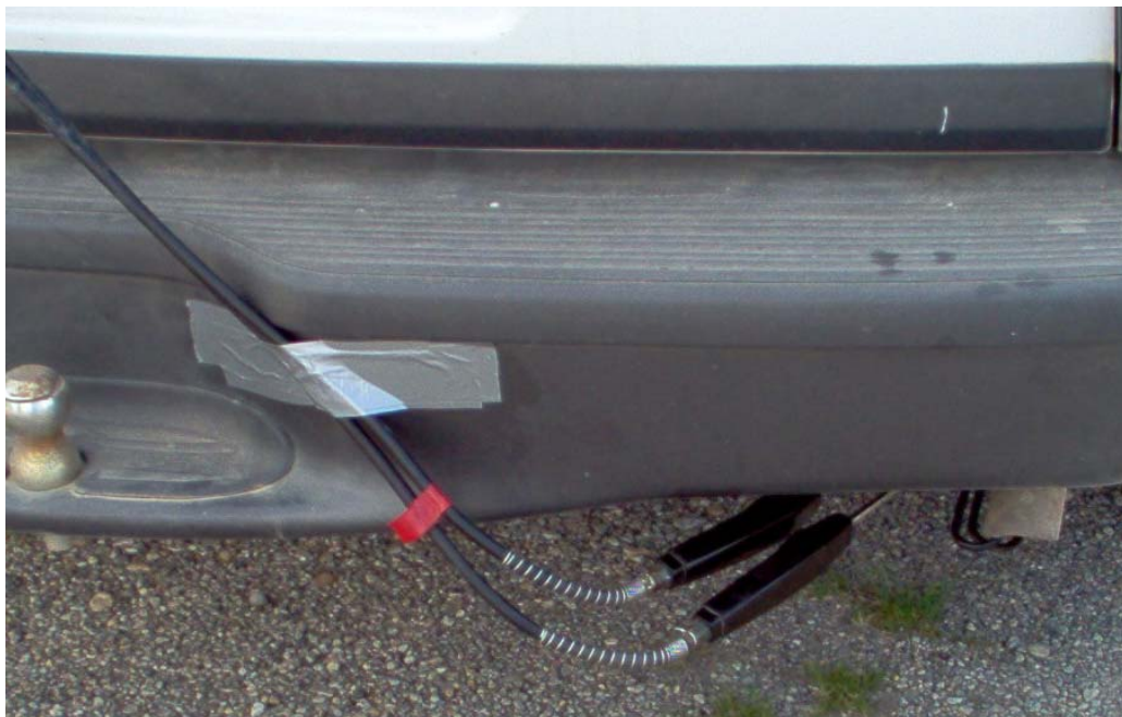
Figure 3. Photos of PEMS Equipment Connected to Test Vehicle.
