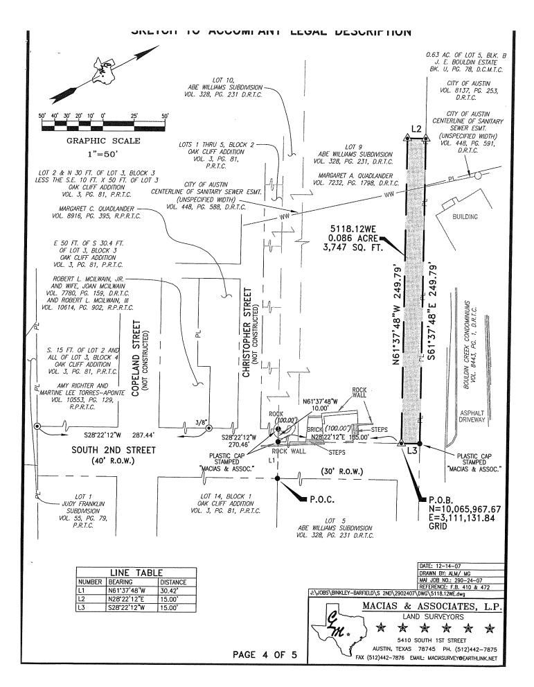
**LEGEND** 1/2" IRON ROD FOUND (UNLESS OTHERWISE NOTED) 1/2" IRON PIPE FOUND ( (UNLESS OTHERWISE NOTED) ◬ 60D NAIL SET Δ CALCULATED POINT P.O.B. POINT OF BEGINNING POINT OF COMMENCEMENT P.O.C. R.O.W. RIGHT-OF-WAY — PL— PROPERTY LINE VOL., PG. VOLUME, PAGE DEED RECORDS OF D.R.T.C. TRAVIS COUNTY PLAT RECORDS OF TRAVIS COUNTY P.R.T.C. DISTRICT COURT MINUTES OF TRAVIS COUNTY D.C.M.T.C. REAL PROPERTY RECORDS OF TRAVIS COUNTY R.P.R.T.C. ( ) RECORD INFORMATION
