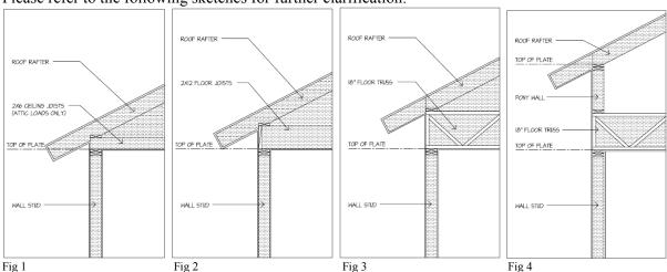
Figures 1, 2, and 3 are examples of acceptable construction methods that would qualify as being "fully contained within the roof structure." Figure 4 is a sketch of an unacceptable construction method for the purpose of qualifying as being "fully contained within the roof structure." This attic area would not qualify for exclusion from the calculation of gross floor area.
