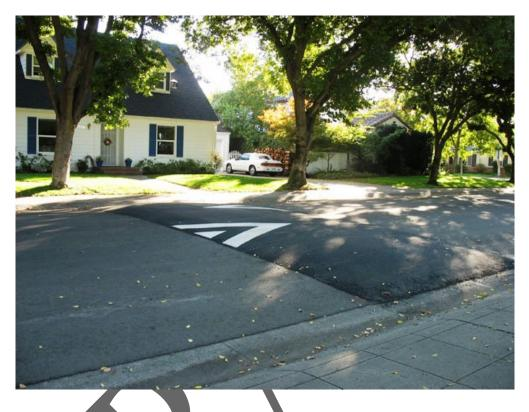
Speed humps are rounded raised areas placed across the roadway. They are generally 10 to 14 feet long (in the direction of travel), making them distinct from the shorter "speed **bumps**" found in many parking lots, and are 3 to 4 inches high. The profile of a speed hump can be circular, parabolic, or sinusoidal. They are often tapered as they reach the curb on each end to allow unimpeded drainage.
