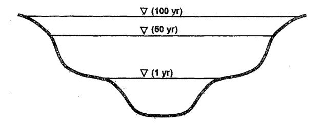
Typical modified channel cross-section. Designer shall ensure longitudinal slope meets non-erosive permissible shear requirements.
