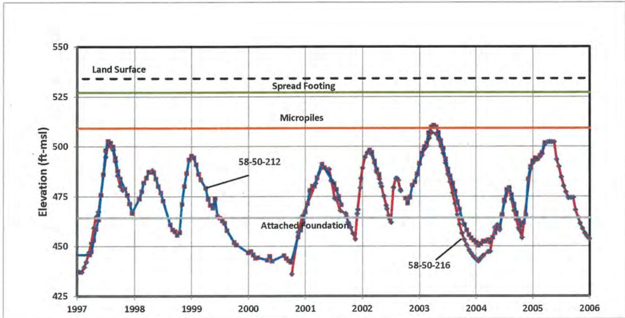
Figure 5. Comparisons of groundwater levels with bottom of penetrations for three foundation alternatives.
