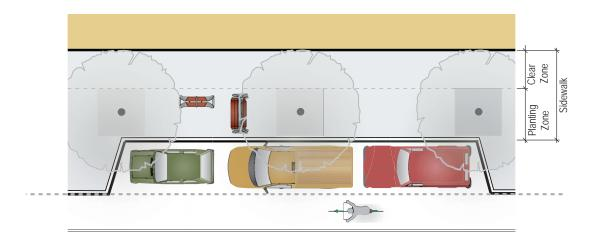
**Figure 3-8:** On-street parallel parking design inside the curb line.
