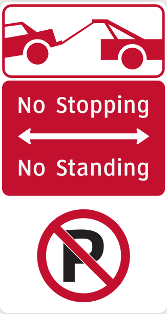
NO PARKING, NO STOPPING, NO STANDING, TOW Finished dimension 30"x12". Curve, kerf and affix to freeway concrete columns at designated locations per sign plan Page 5 of this document. No straps or bolts shall be visible. If hidden connections are not feasible, vendor may affix with epoxy, resin, 3M dual adhesive or other product which must carry a warranty and be approved by both architect and FÖDA Studio.
