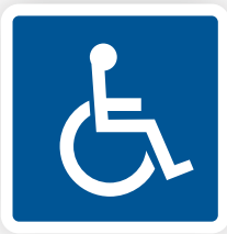
ACCESSIBLE Freestanding signs at marked locations on plan. Finished dimension, 8"x8", mounting height as per city guidelines on standard sign mounting poles and substrate.
