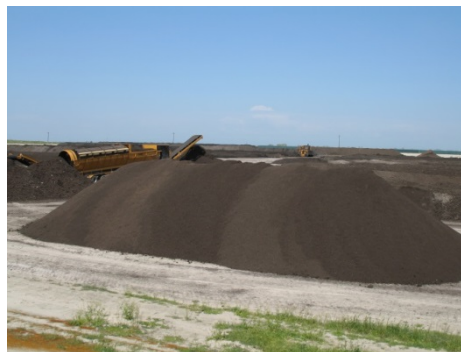
At our Central Valley Composting facility, Synagro utilizes a mobile chip and grind operation for inbound feedstock size reduction.
