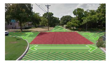
At the above intersection no crosswalk is marked. However, 'unmarked crosswalks' still exist (as highlighted in the arrows) up to the line of the Right-of-Way.
