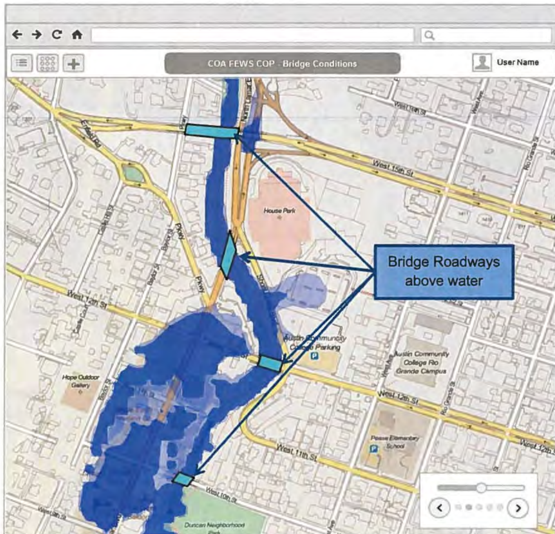
Figure 12 Inundation map showing bridges that are above/below water surface elevation based on low/high chord elevations
