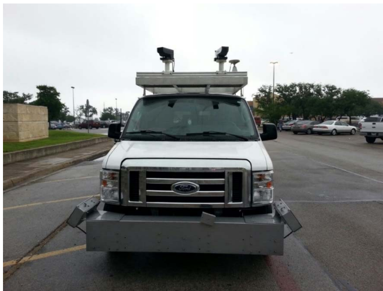
DTS MAC vehicles feature 5 laser profilers
