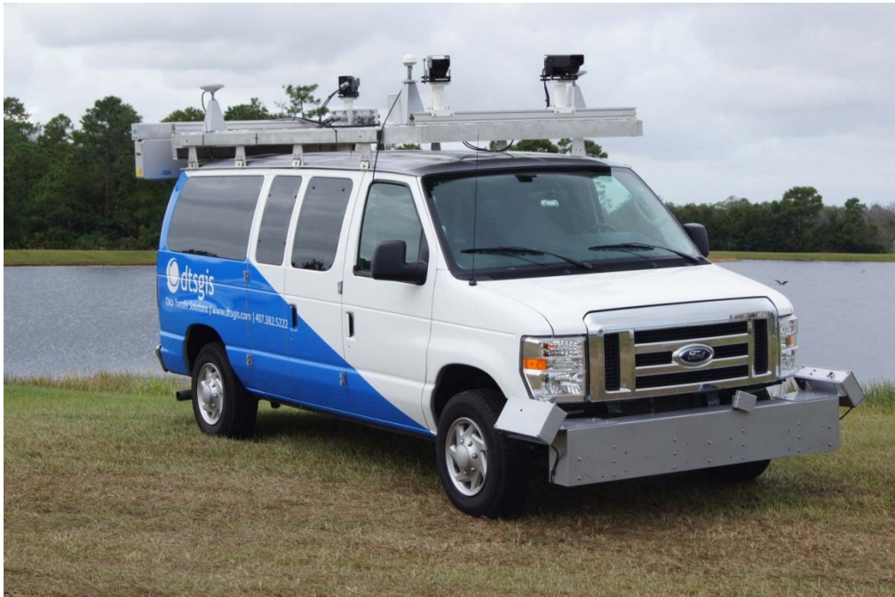
Mobile Asset Collection Vehicle with Profiling Equipment per Specification and Certified by TTI
