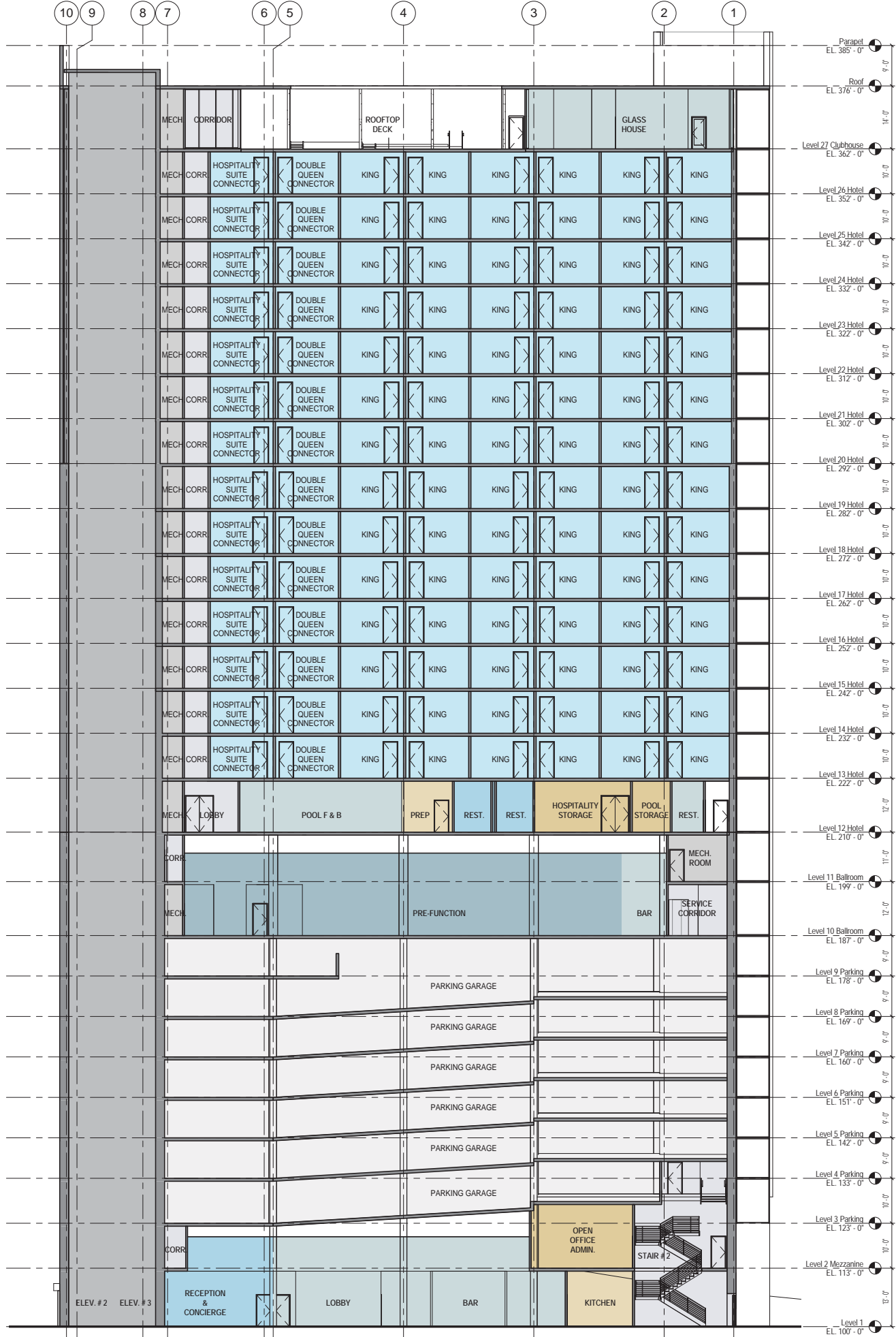
BUILDING SECTIONS THROUGH 02 CIRCULATION SCALE: 3/32" = 1'-0"
