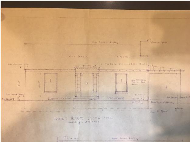
Blueprint showing the original configuration of the front porch. The applicant proposes to reconstruct the porch in accordance with this drawing.
