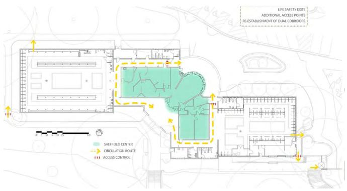
**Bathhouse Projects, Phase One:** Rehabilitation of the Bathhouse will necessitate a phased plan of improvements in order to minimize disruption during the construction period. The initial project phase should address life-safety concerns pertaining to the Bathhouse and the pool enclosure.
