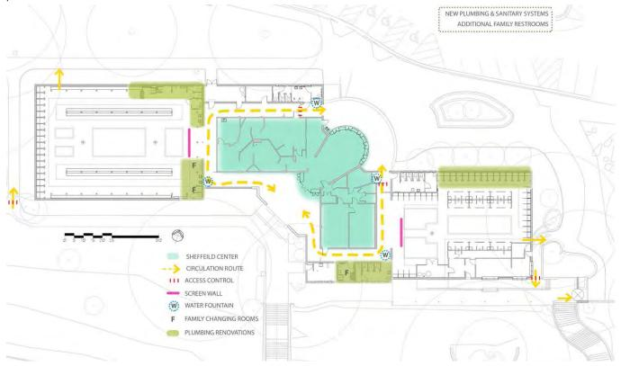
**Bathhouse Projects, Phase Two:** The second project phase should address rehabilitation of existing plumbing systems and the installation of new amenities such as drinking fountains and gender-neutral changing rooms.
