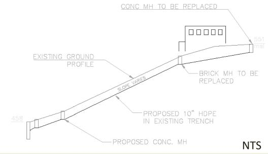
Replacement Option 2 Horizontal Directional Drilling (HDD)
