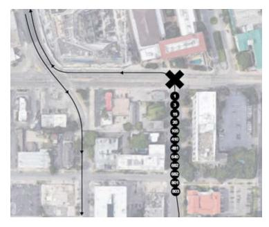
Severe bus delay occurs at Lavaca & MLK Blvd. due to cars interfering with the bus queue (signal).
