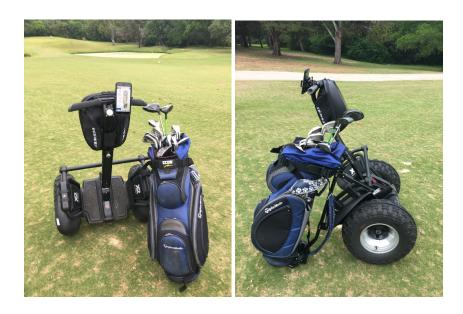
Segway's® revolutionary balance-control system works in tandem with a pair of electric motors, one powering each wheel. It uses brushless DC electric motors powered by lithium-ion batteries using tilt and gyroscopic sensors.
