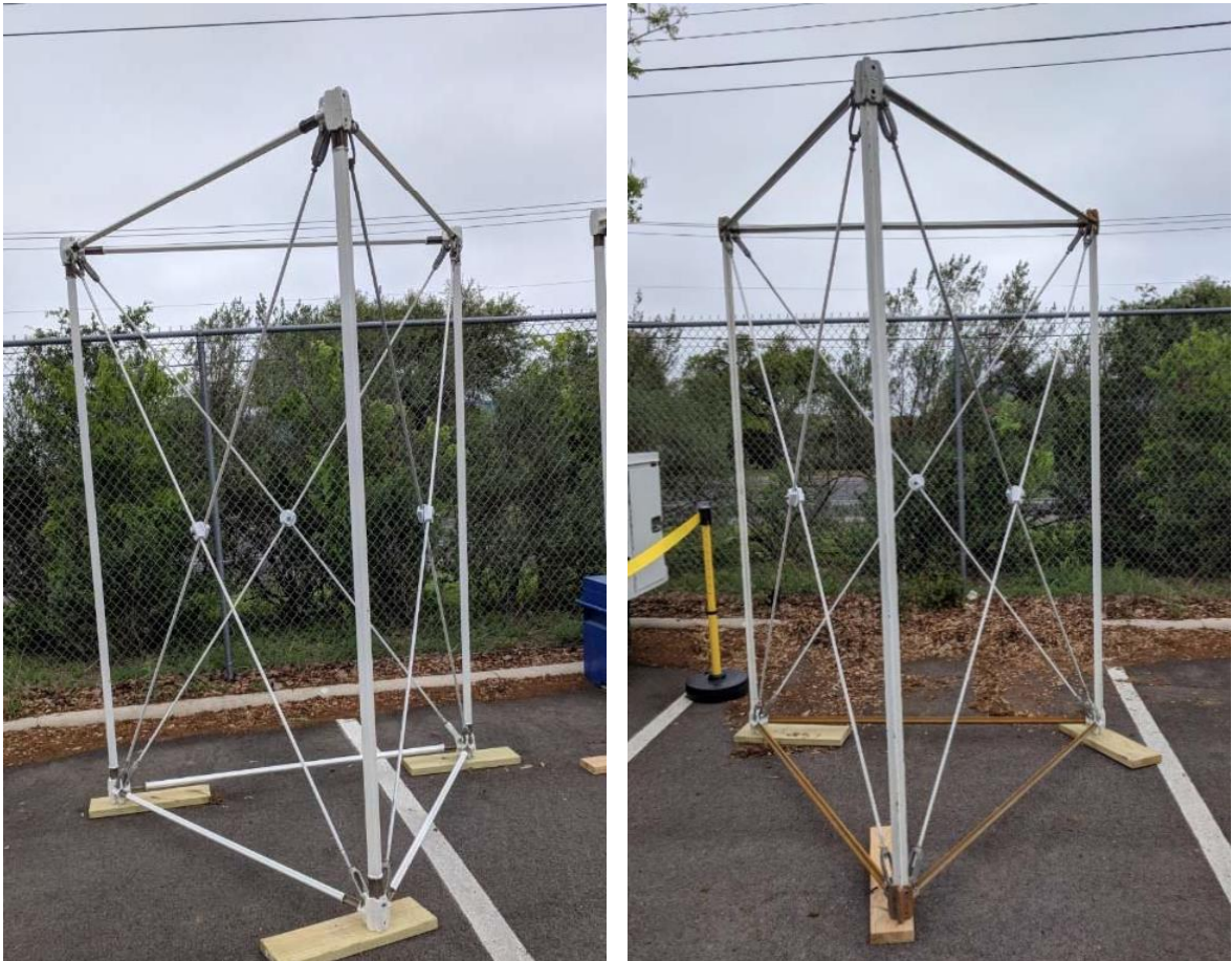
As viewed from 6 feet away: Square tubes (left); original tower section (right)
