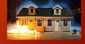
Appendages and structures (decks and fences) attached to or within 10' of structure to be fire resistant except fence materials beyond 10'
