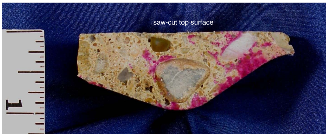
Fig. 4 Saw-cut, cross-sectional concrete surface of Core No. 3-C14. Phenolphthalein (a pH indicator solution) was applied to the surface to aid in carbonation assessment. Non-carbonated paste is deep magenta; carbonated paste did not change color. The majority of the paste is carbonated throughout the full depth of the concrete sample. A small amount of non-carbonated paste is present along the bottom surface and mottled upwardly into the concrete. Scale is in inches.
