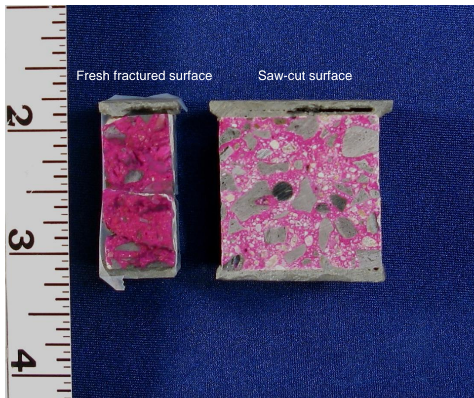
Fig. 1 Core FS#22-C12, after being saw-cut longitudinally in the Petrographic Laboratory. One resultant longitudinal saw-cut surface is shown on the right. The other longitudinal saw-cut surface was freshly fractured in the laboratory (left). Phenolphthalein (a pH indicator solution) was applied to these surfaces to determine localities of paste carbonation in the concrete. Non-carbonated paste is deep magenta; carbonated paste does not change color. In the core specimen, no carbonation is observed. Scale is in inches.
