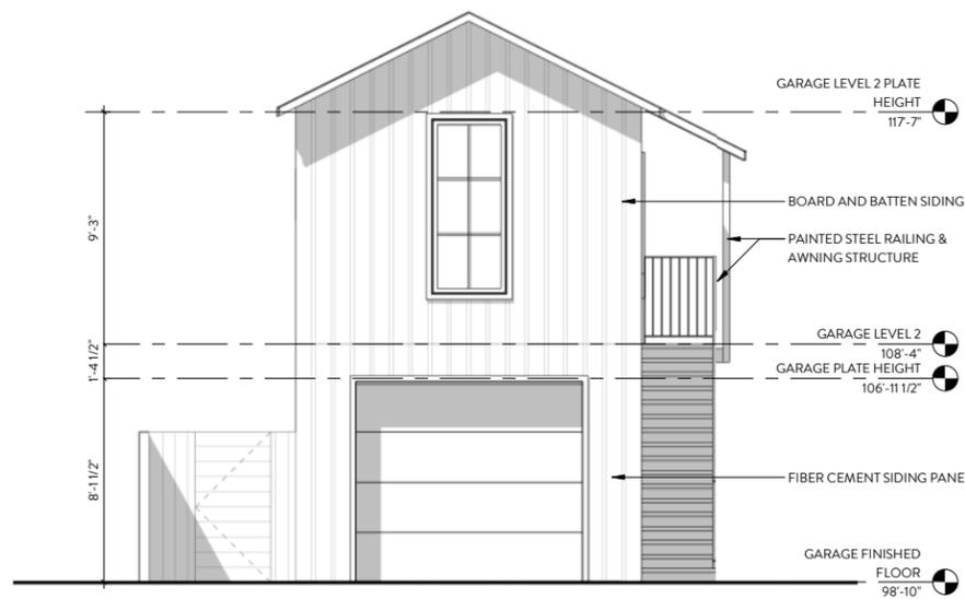
**GARAGE - PROPOSED SOUTH ELEVATION**
