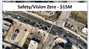
Improvements on Oltorf at Parker include new medians, high-visibility crosswalks, ADA accessible curb ramps, a shared use path, and relocated bus stops. This is the 12<sup>th</sup> completed intersection.
