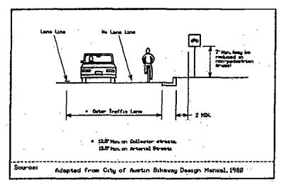
Schematic drawing of a bicycle compatible street
