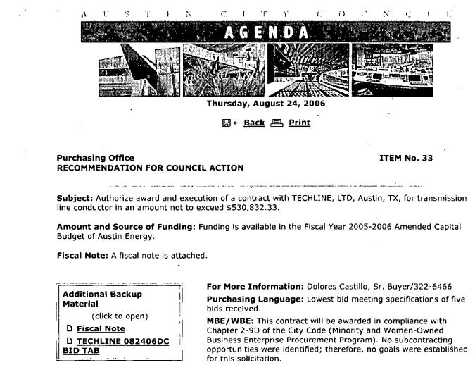
This contract will provide Austin Energy with 273,120 pounds of transmission line conductor. This conductor is required to re-conduct transmission line circuits 138kV, Ckt 1021, Kingsberry to Bergstron Substations and 69kV Ckt 822, Cardinal Lane to Burleson Substation. The transmission line conductor is required to increase transmission capacity. This increased capacity will preclude overloading under contingency conditions.
