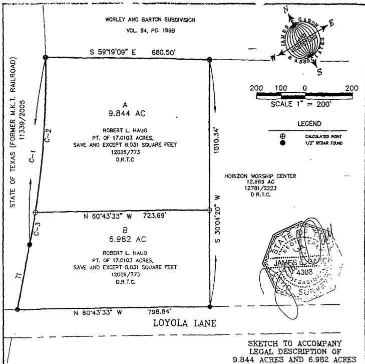
TANGENT BEARING LENGTH N 41"01'26" E 274.94 T1 DELTA BEARING CURVE RADIUS LENGTH CHORD NJ5'02'56"E 761.64' 3658,70' 763.02' 11'56'55" C-1 09'51'48" S34'00'24"W 629.06" C-2 3658.70' 629 83' 02'05'10" S39'58'53"W 133.21' C-33658.70' 133.22'
