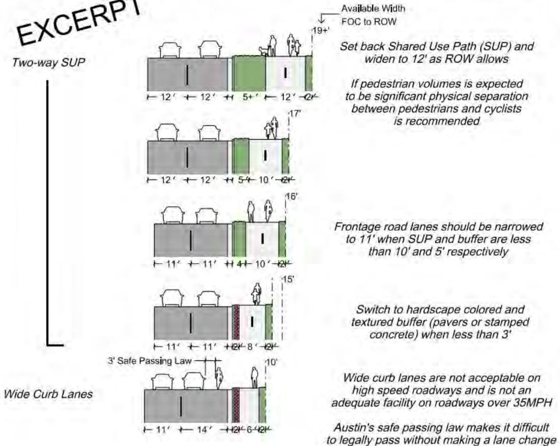
**EXCERPT FROM FULL GUIDANCE ON RECOMMENDED BICYCLE AND PEDESTRIAN FACILITIES ALONG HIGH SPEED ROADWAYS WITH LIMITED ACCESS DEVELOPED BY THE CITY OF AUSTIN IN COORDINATION WITH THE TXDOT AUSTIN DISTRICT.**
