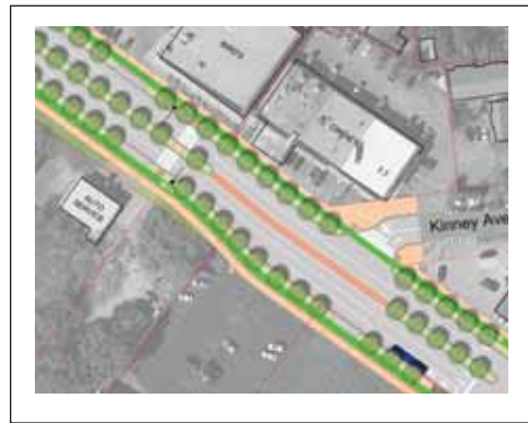
Raised median with paved center turn lane at Kinney Avenue.
