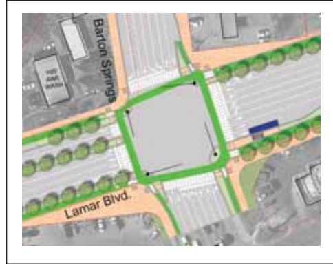
A second left turn lane will ease queuing at Barton Springs Road.
