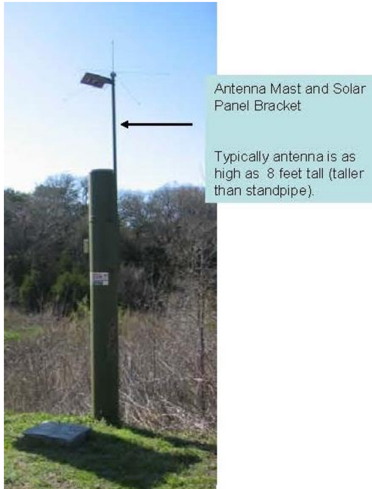
A typical rain gauge
