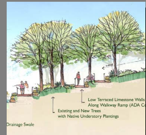
Section – South Woods ADA Trail Min. Width 5'-6"
