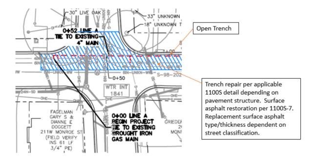
For Concrete pavements, concrete restoration limits are determined by joint locations.
