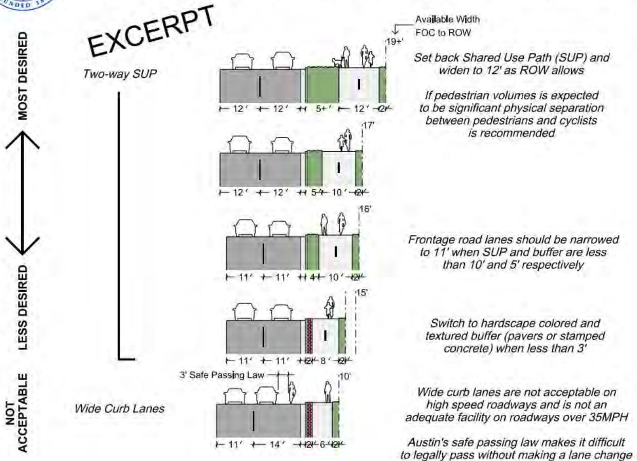
**EXCERPT FROM FULL GUIDANCE ON RECOMMENDED BICYCLE AND PEDESTRIAN FACILITIES ALONG HIGH SPEED ROADWAYS WITH LIMITED ACCESS DEVELOPED BY THE CITY OF AUSTIN IN COORDINATION WITH THE TXDOT AUSTIN DISTRICT.**
