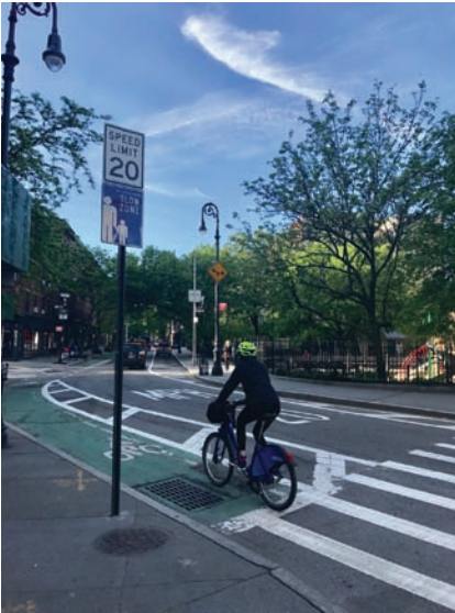
A Slow Zone in New York City uses lower speed limits, special signs, and street design to reduce vehicle speeds.
