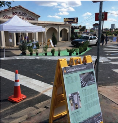
Demonstration bulbout (green pavement) and education sign at the Burnet Road Better Block.
