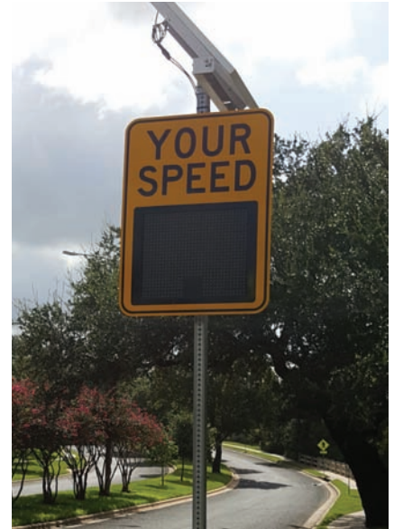
Dynamic Speed Display Devices provide people driving real-time speed feedback to alert people exceeding the speed limit.
