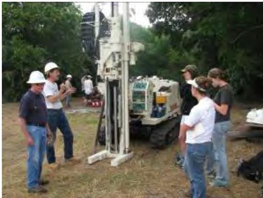
Geoprobe soil core samples being taken on Platt 4 field June 2007
