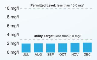
Ensure stream water quality by keeping the Carbonaceous Biological Oxygen Demand (CBOD) concentration from our wastewater treatment plants discharges at 3.0 mg/L or less.
