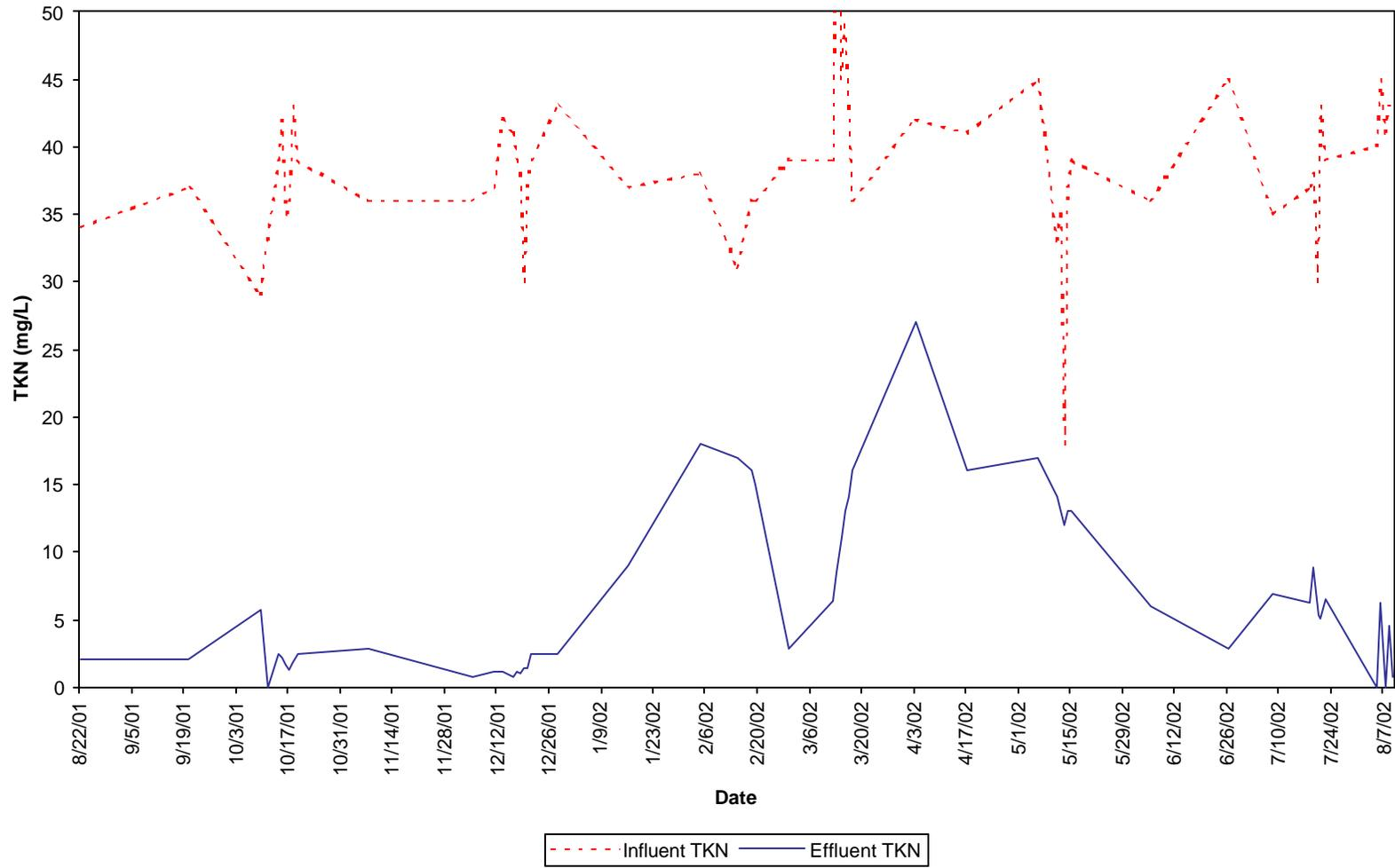
**Figure 4-3. SeptiTech® Model 400 System Total Kjeldahl Nitrogen Results**
