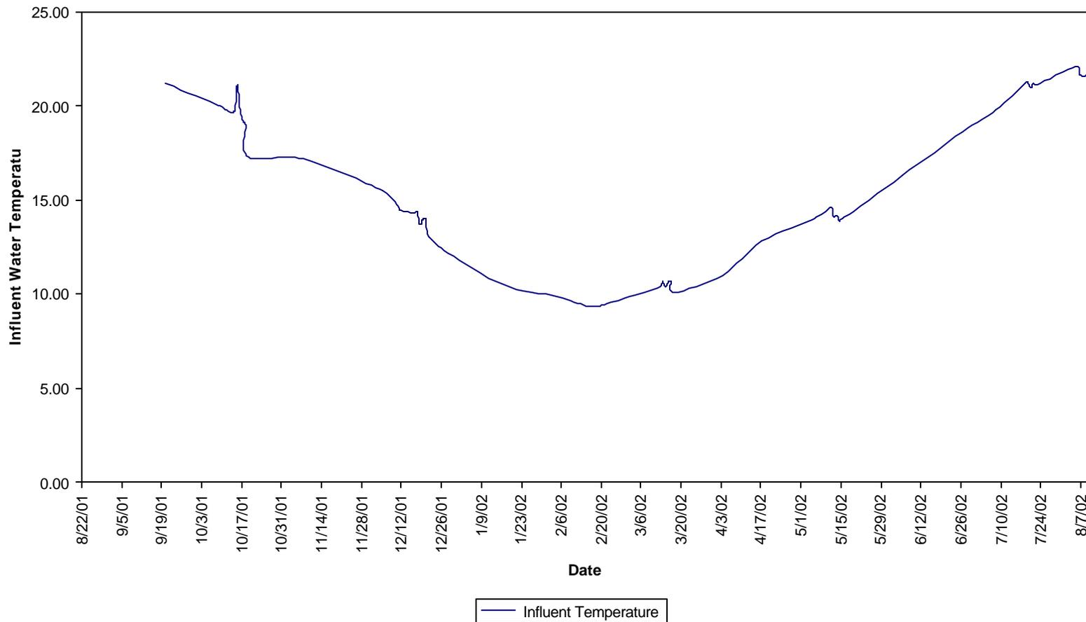
**Figure 4-7. SeptiTech® Model 400 System Influent Temperature**
