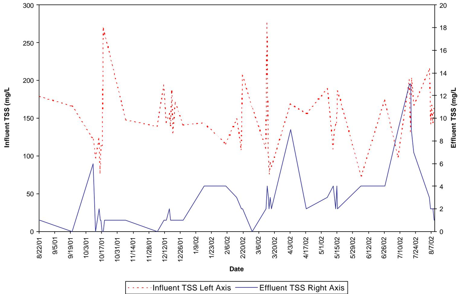
**Figure 4-2. SeptiTech® Model 400 System Total Suspended Solids Results**
