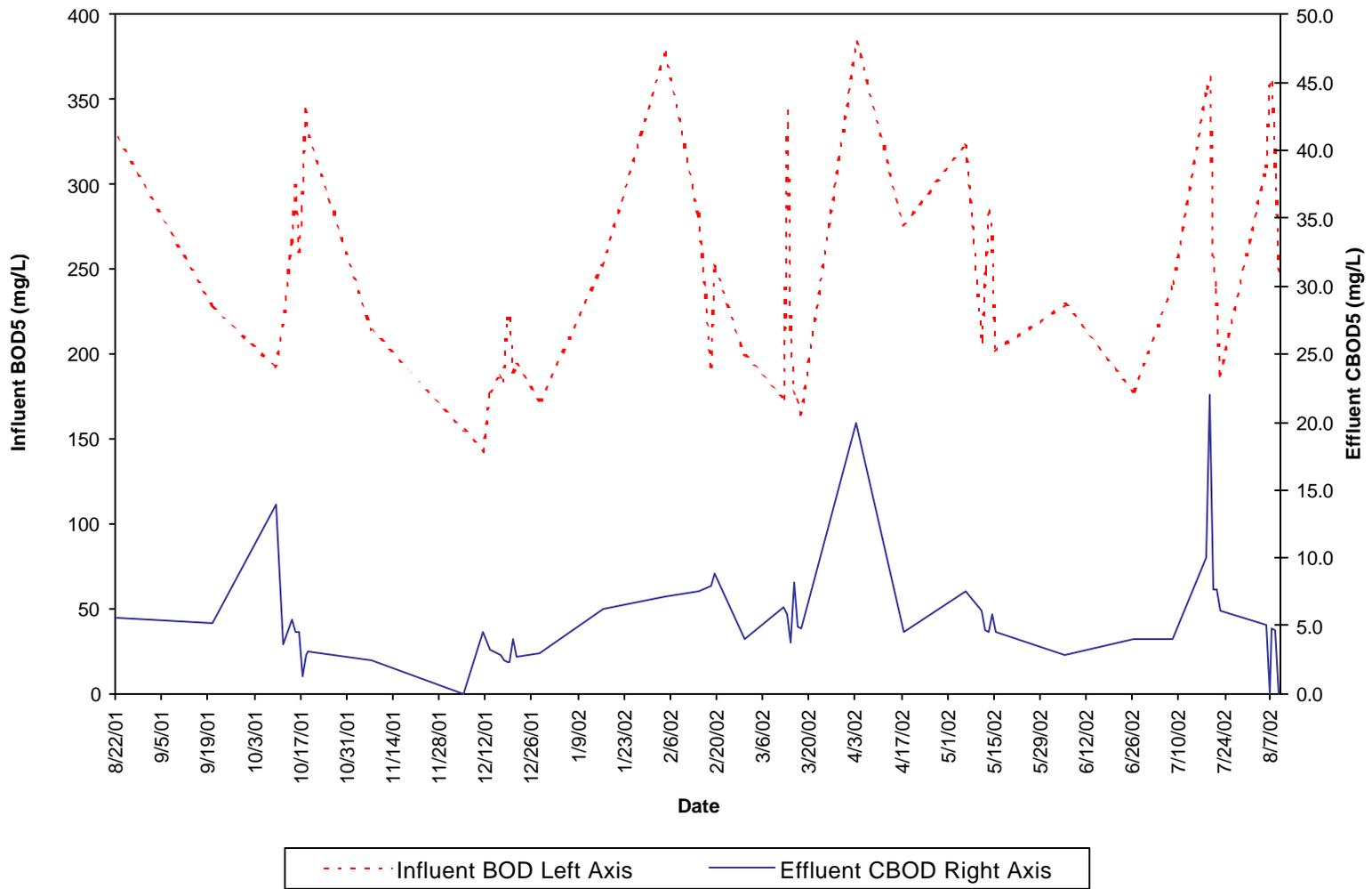
**Figure 4-1. SeptiTech® Model 400 System BOD<sub>5</sub>/CBOD<sub>5</sub> Results**
