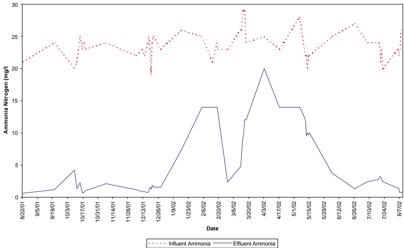
**Figure 4-4. SeptiTech® Model 400 System Ammonia Nitrogen Results**
