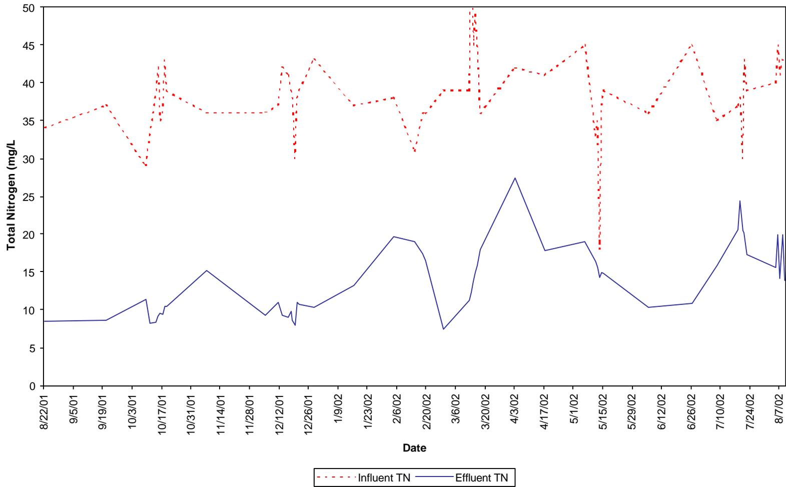
**Figure 4-5. SeptiTech® Model 400 System Total Nitrogen Results**
