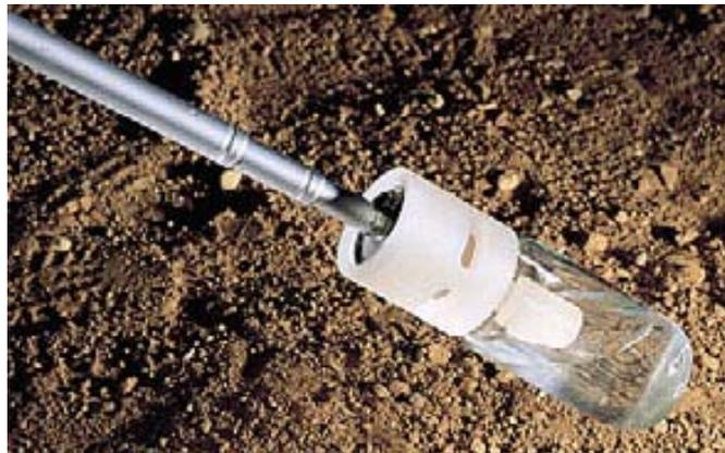
**Figure 2-1. Subsurface grab sampler.**
