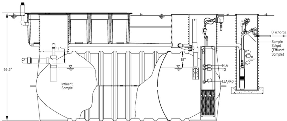
**Figure 2-2. Sampling arrangement.**
