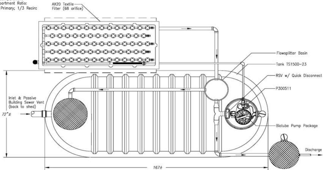
**Figure 1-5. Plan view of treatment system layout.**
