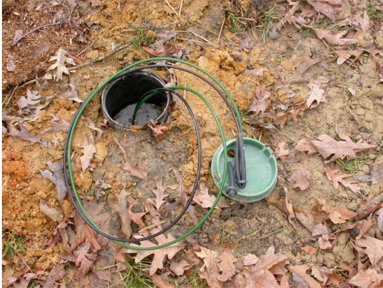
**Photograph 3: Completed Lysimeter Installation with Sampling Tubes Exposed**
