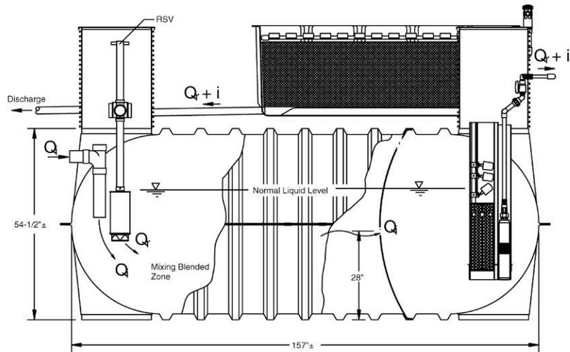
**Figure 5: AdvanTex Mode 3 – Profile View**
