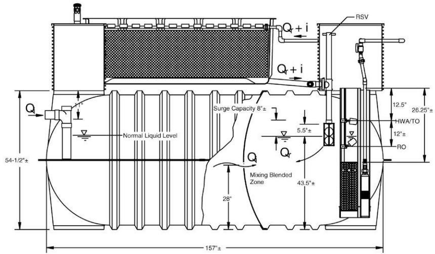
**Figure 3: AdvanTex Mode 1 – Profile View**
