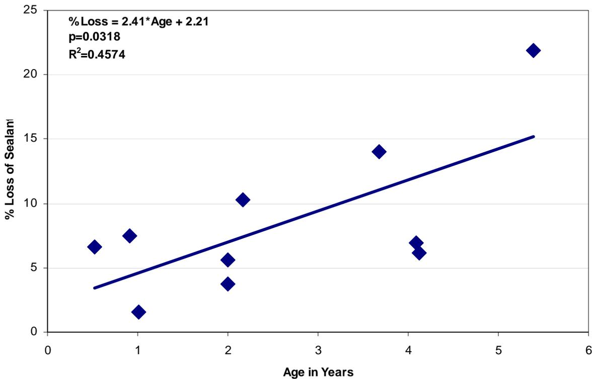
Figure 7. Linear relationship between sealant loss and age of sealant.
