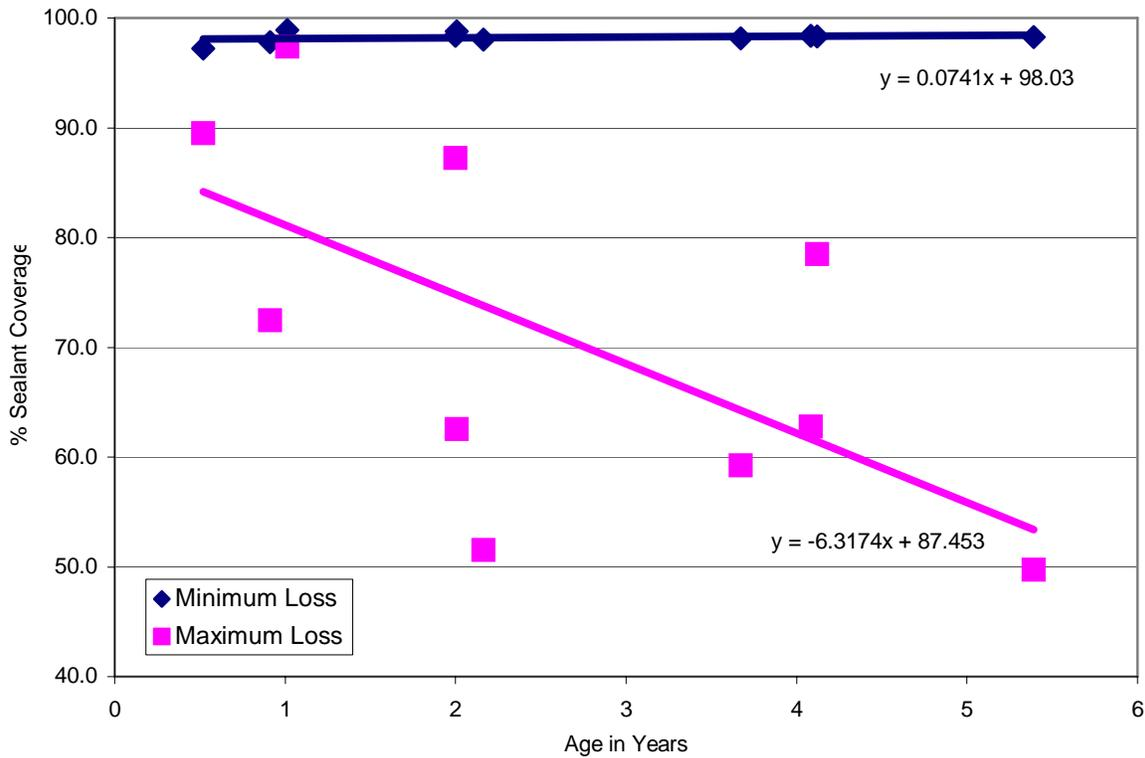
Figure 5. The observed minimal (blue) and maximal (pink) sealant wear as a function of age in years.
