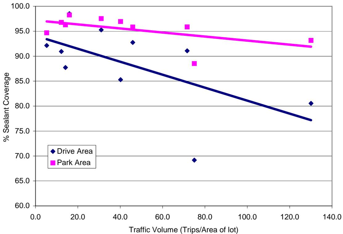
Figure 6. Sealant remaining in drive areas and park areas as a function of traffic volume.
