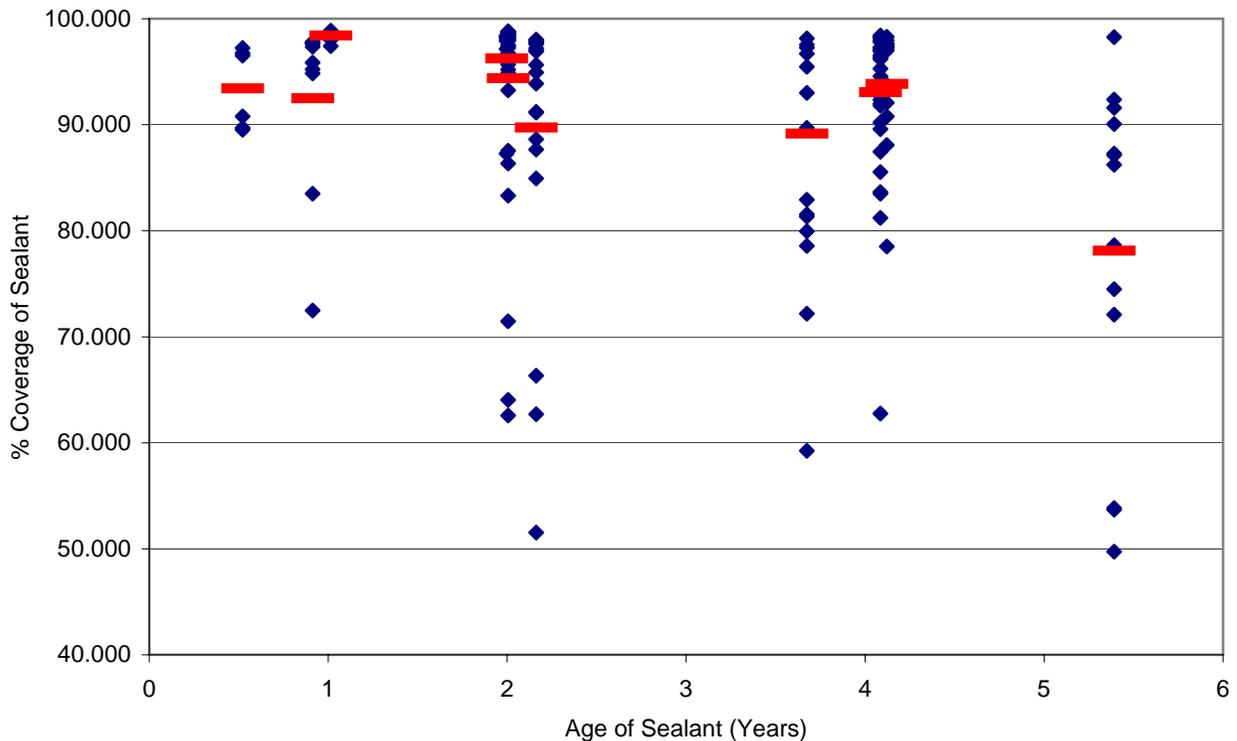
Figure 4. Percent sealant remaining on 10 study parking lots as a function of age in years. The vertical lines of data points (diamonds) represent all data from each of the study lots. The lateral red bar represents the average amount of sealant on each lot at the time the photographs were taken.
