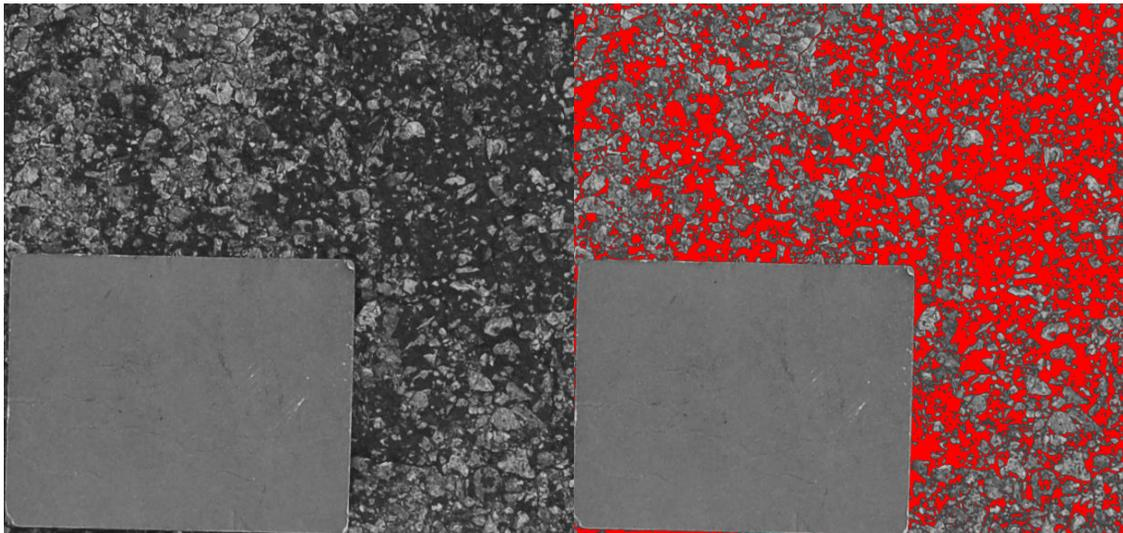
Figure 3. Example of density slicing technique of separating sealant from unsealed asphalt. The photo on the left shows a black and white image where black=sealant, while the photo on the right shows the separation of sealant from background, using false red color.
