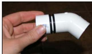
Same picture as above with another #18 O-Ring and the  $\frac{3}{4}$ " 45° elbow added. Note: the coupler and one O-Ring should be on the inside of the container and the other O-Ring and  $\frac{3}{4}$ " 45° elbow should be on the outside of the container. All parts should be pressed together tightly to make a watertight seal.
