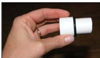
$\frac{3}{4}$ " PVC tubing with #18 O-Ring (black) and coupler cut in half (on left).
