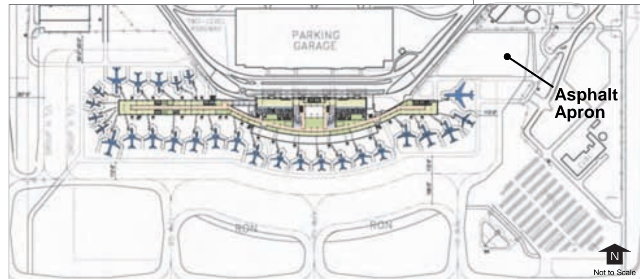
Figure 4 Existing Passenger Terminal and Apron Configuration
