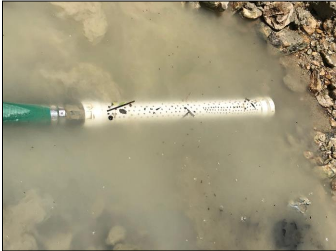
Figure 6. A baffle must be placed over the pump intake to stop even small fish from being drawn into the pump
