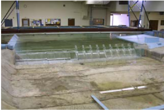
Hydrodynamic models can be physical scale models like this, or they can be numerical (computer) models. In slow moving waters, like those of Barton Springs, the sensors on a physical model are unable to make accurate detections.
