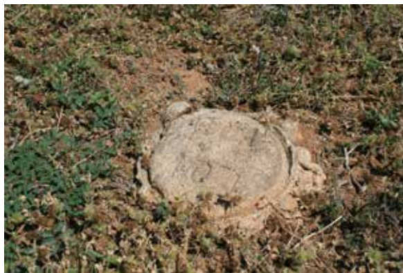
Figure 412. Ground-level concrete markers identify plot corners. (John Milner Associates )
