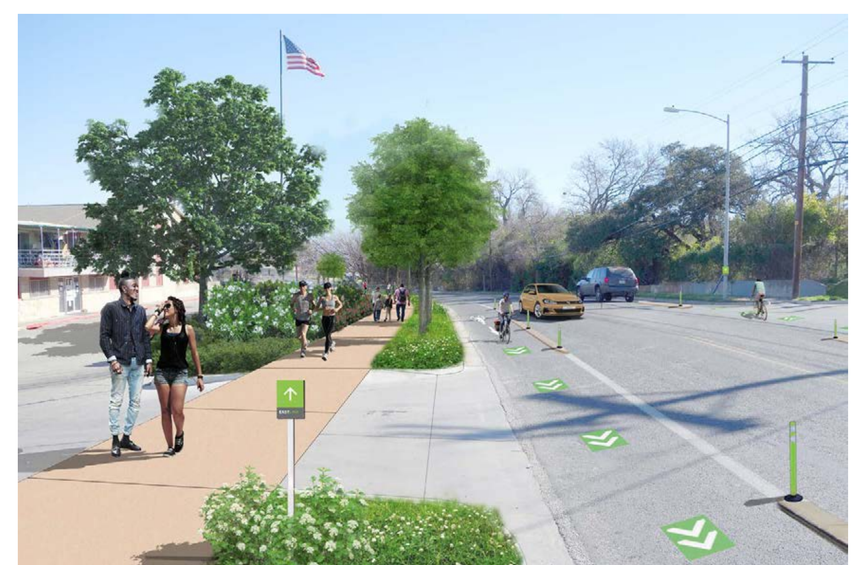
C Future view of Manor Rd with wider sidewalk on north side and protected bicycle lanes, looking east
