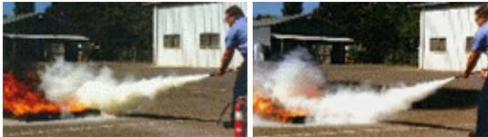
**Sweep** the nozzle back and forth at the base of the fire. After the fire appears to be out, watch it carefully since it may re-ignite!
