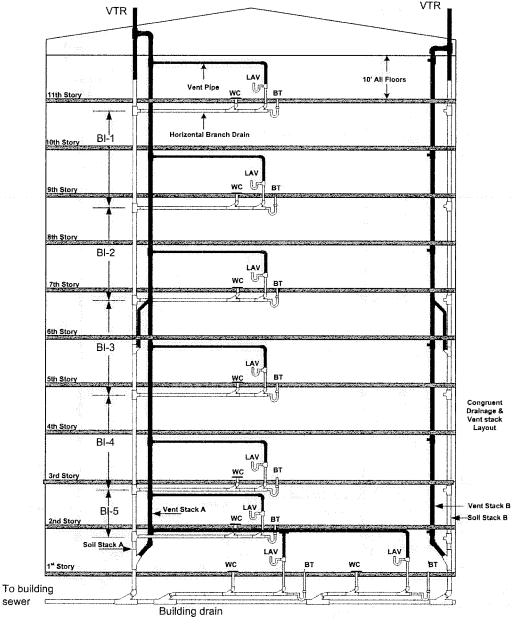
Note: Horizontal branch drain, vent pipe & AAV's serving bathrooms and connecting to vent & soil stack B are not shown but have an identical layout of those shown connecting to vent & soil stack A.
